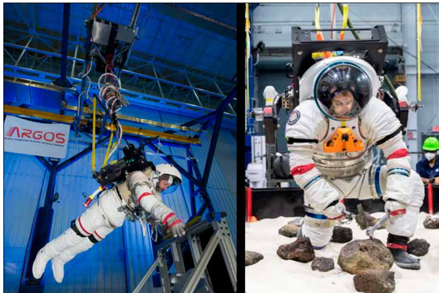
FIGURE 2 Testing to characterize crewmember capabilities and constraints in spacesuits often uses test environments such as the Active Response Gravity Offload System (ARGOS) shown here, which allows for simulation of reduced-gravity EVA conditions using a system similar to an overhead bridge crane.
