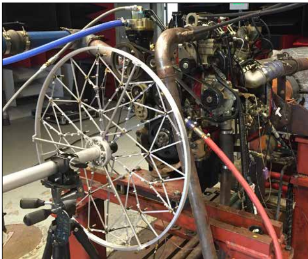
FIGURE 2 Typical modern microphone array for acoustic source localization. This array features 36 microphones and is being used to identify noise source locations on the front of a diesel engine. Photograph courtesy of Tongyang Shi.
