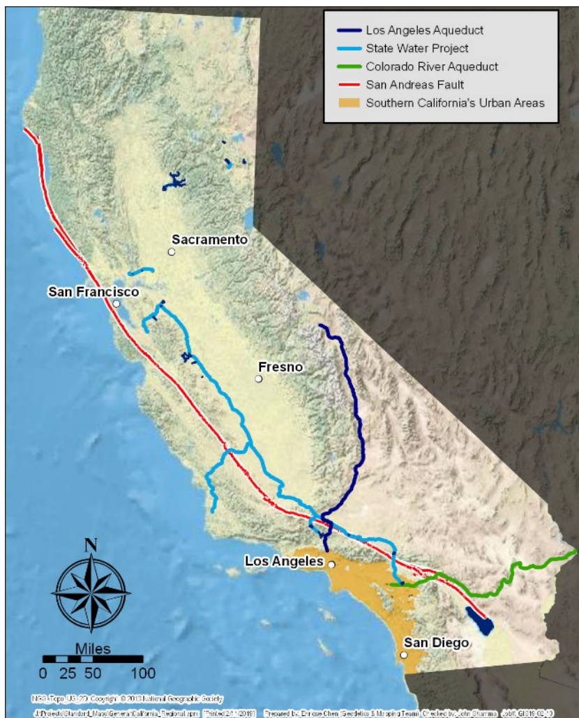
FIGURE 1 Major aqueduct systems that import water to Southern California. The legend identifies each aqueduct, the San Andreas Fault, and the Southern California urban area. All three systems, which provide water to the Los Angeles and San Diego urban area, cross the San Andreas Fault (red line).
