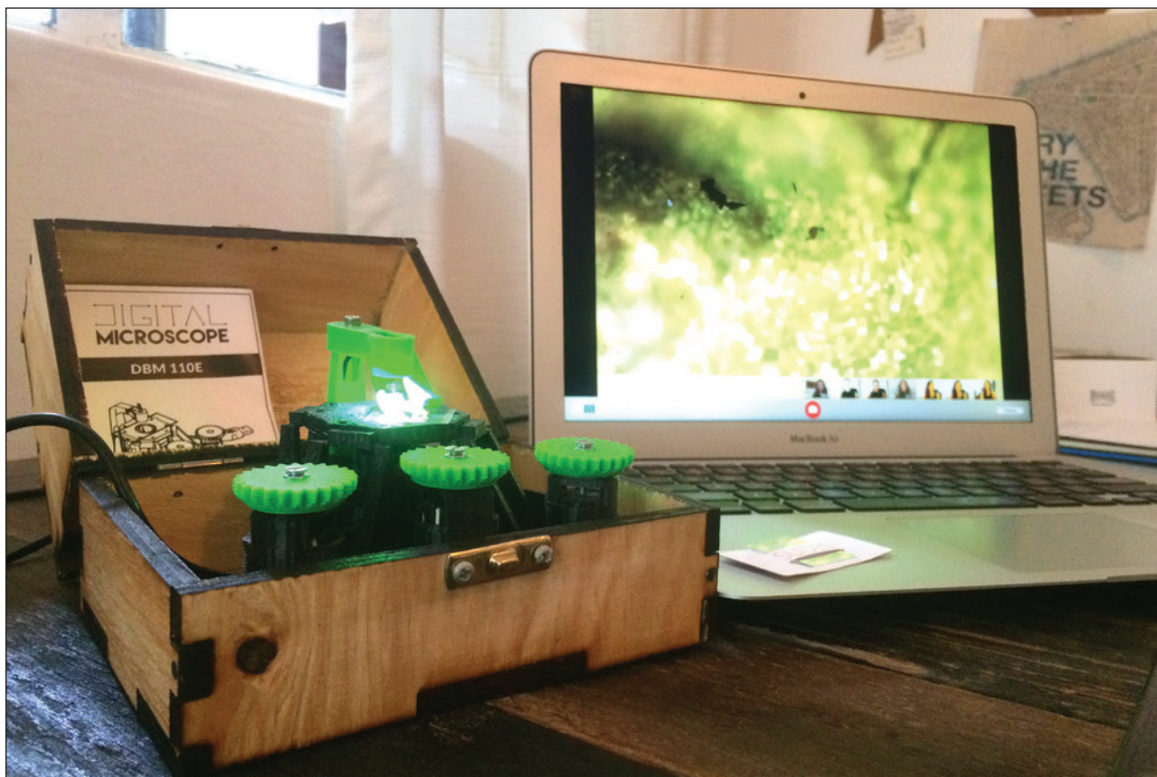
FIGURE 4 Open flexure microscope (left) made in Nairobi using Retr3D printers. Microscope view is projected on the laptop screen.
