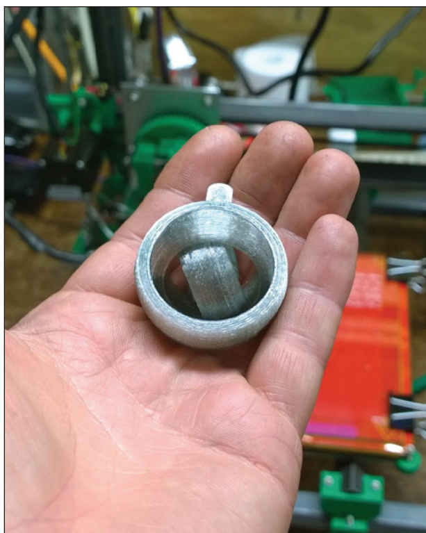
FIGURE 3 Keychain printed with recycled polyethylene terephthalate (PET) filament made with the Thunderhead filament extruder and printed using a Retr3D printer.
