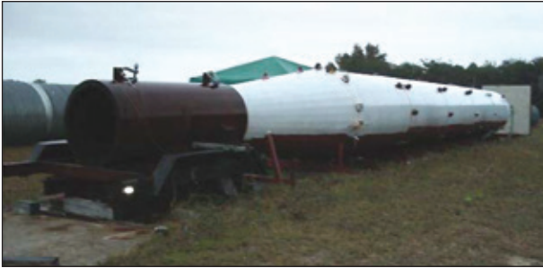
FIGURE 1 Blast wave generator. Photo credit: USUHS Neurotrauma Laboratory.
